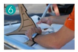
Once the piece is in place and backing paper fully removed press down on the entire surface to ensure bond. Now take your roller and roll in a back and forth motion from the center of the piece, working your way to the outside. Apply even pressure. If you get a small bubble that will not work itself out you can poke a hole in the mat with a pin or the point of your razor knife and push the air out through the hole. The hole will be invisible once it is pressed down.
