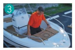
Lay all pieces into their proper area for installation and check for fit and alignment. Once you are happy with the fit it is time to install. We suggest beginning at either the front or back and working towards the other direction.
