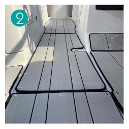
Lay all the mats in the proper location on the cockpit floor. Take care to align all the edges and pattern lines for one continuous look.
