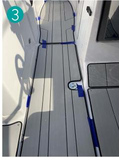
Using the masking tape, tape all the pieces into place to temporarily hold them while installing the studs into the deck of the boat.
