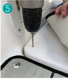
Lift the corner or edge of the mat and drill the final hole for the stud with the 1/8" drill bit.
