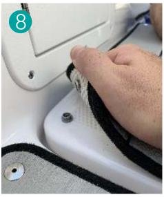
Repeat steps 4-7 for all remaining snaps being careful to make sure the mats stay aligned and are laying flat before drilling each hole.
