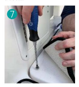
Using the screwdriver, tighten the snap stud through the washer in the hole and snap the mat to it.
