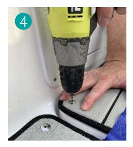
Your new patented Marine Mat Snap-it Series mats utilized a unique drill guide snap cap. These snaps have a pilot or guide hole to allow for perfect alignment every time. Working from the front of the boat to the rear use the 1/16" or 7/64" drill bit, drill your first pilot hole through the guide in the snap itself into the deck of the boat.
